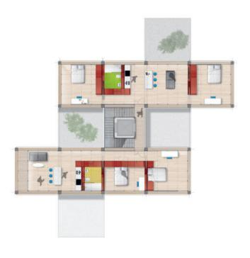
The units are stacked, using a simple gravity structure, around a central stair and lift. Minimal foundations are required.
