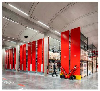
A post-beam construction system on an 8 by 10-metre grid offers great flexibility of use as well as a certain modularity. The workspaces are separated from the reserves by a top-lit central corridor – the internal 'artworks boulevard' of the building and its principal circulation space.
